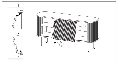
**STEP16**: Insert the Door Right (L) into the upper groove line, hold then align the lower side of door to properly placed inside the bottom track.
