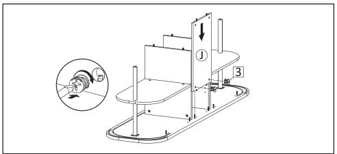
**STEP6**: Attach Back Board 2 (J) into Top Board (A). Insert Camlock (HW3) then tighten using screwdriver.
