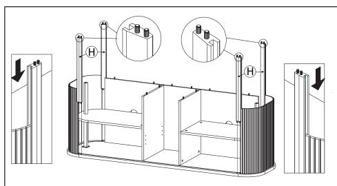
**STEP9**: Insert Support Board (H) into Top Board. Please notice the grooved side must be placed facing the Bar Side.
