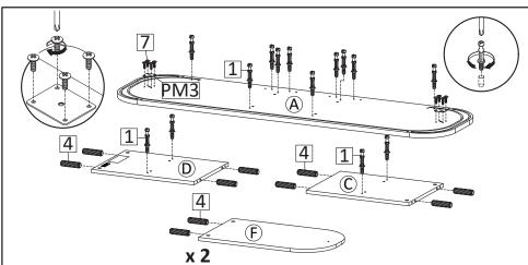
**STEP1**: Insert Cambolt (HW1) into Top Board (A), Center Board Left (C) and Center Board Right (D). Insert Mounting Plate (HW PM3) to Top Board (A) secure with Screw M4.5x12.5mm (HW7). Insert Dowel Big (HW4) into Fixed Shelf (F).
