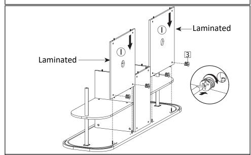
**STEP7**: Attach Back Board 1 (I) into Top Board (A). Insert Camlock (HW3) then tighten using screwdrive as figure.
