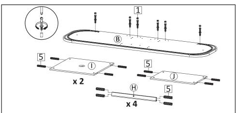
STEP2: Insert Cambolt (HW1) into Bottom Board (B). Insert Dowel Small (HW5) into Support Board (H) and Back Boards (I&J) as figure.
