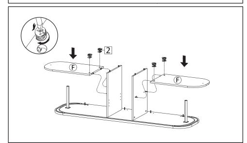
**STEP4**: Attach Fixed Shelf (F) into Center Boards. Insert Camlock (HW2) then tighten using screwdriver as picture.
