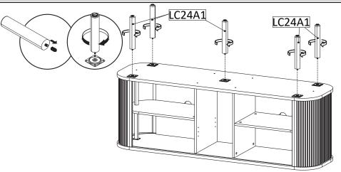
**STEP12**: Install Leg (LC24A1) into Mounting Plate, tighten by rotating the leg clockwise.
