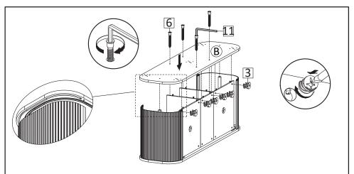
**STEP10**: Place Bottom Board (B) onto main assembled unit. Ensure the Bar Side has been properly inserted into the outer groove line of the Bottom Board.Use Screw M7x50mm (HW6) to secure Bottom Board, tighten screws using Allen Key (HW11) as figure. Insert Camlock Small (HW3) to Back Board then tighten using screwdrive as figure.
