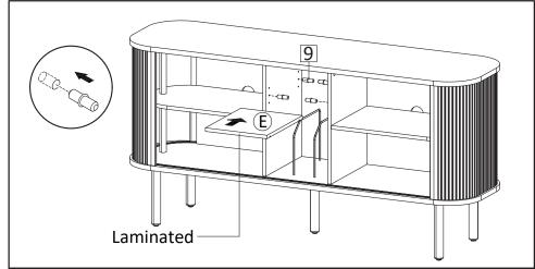
**STEP14**: Insert Shelf Pin (HW9) into the holes on Center Boards, on the desired level. Then place the Adjustable Shelf (E) onto shelf pin.
