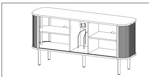
**STEP13**: Insert Divider Wire (HW13) into Bottom Board, ensure the wire has been properly inserted into the provided hole.
