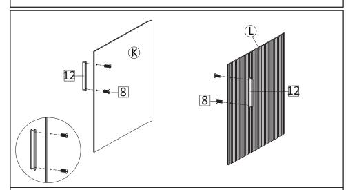
**STEP15**: Insert Handle (HW12) into the holes on Doors (K&L), secure with Screw M4x10mm (HW8).
