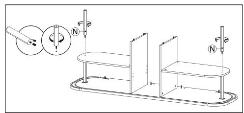
**STEP5**: Insert Pillar 2 (N) into Top Board position as the above image.
