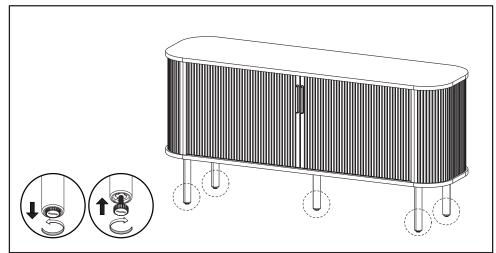
**STEP18**: Place your furniture on lever floor. The legs come with adjustable leveler, adjust it as needed until your furniture stands steadily on the floor. Assembly is Complete.
