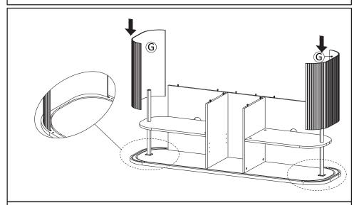
**STEP8**: Carefully insert Bar Side (G) into Top Board outer groove line as above image.
