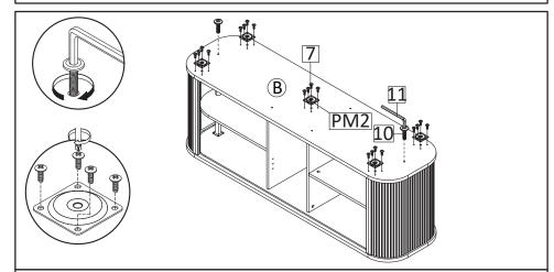
**STEP11**:Insert Screw M6x30mm (HW10), tighten using Allen Key (HW11) to secure Pillar (N). Install Mounting Plate (HW PM2) and secure with screw M4.5x12.5mm (HW7) on Bottom Board.
