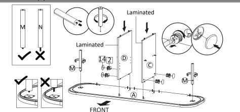
**STEP3**: Attach Center Boards (C&D) into Top Board (A) with laminated edge facing front. Insert Camlock Big (HW2) then tighten using screwdriver. Put Screw Cap (HW14) over the camlock. Pillar 1 (M) has shorter bolt compare to Pillar 2 (N). Please make sure install correct Pillar (M) into the Mounting Plate, tighten by rotating clockwise.
