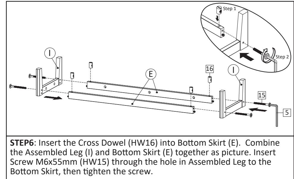
**STEP6:** Insert the Cross Dowel (HW16) into Bottom Skirt (E). Combine the Assembled Leg (I) and Bottom Skirt (E) together as picture. Insert Screw M6x55mm (HW15) through the hole in Assembled Leg to the Bottom Skirt, then tighten the screw.
