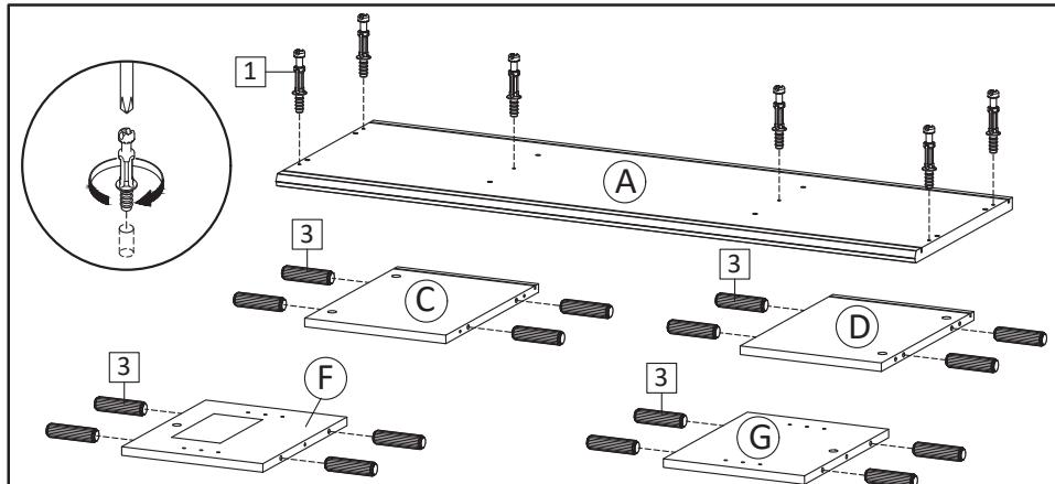
**STEP1:** Insert Cambolt (HW1) into Top Board (A) . Insert Dowel (HW3) into Side Board Left & Side Board Right (C&D) and Center Board Left (F), Center Board Right (G).
