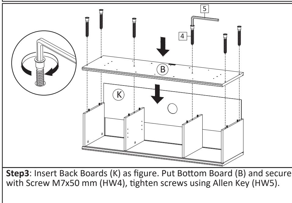
**Step3:** Insert Back Boards (K) as figure. Put Bottom Board (B) and secure with Screw M7x50 mm (HW4), tighten screws using Allen Key (HW5).
