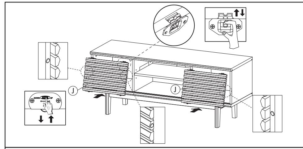
**Step12:** Install the door by inserting the Sliding Top (HW9) pin into the groove line of Top Board. Position the Sliding Bottom (HW10) into the grooved sliding track. Adjust gap of the door,by scroll the button on Sliding Roller (HW10). Follow the down and up direction. Slide the door to right and let ensuring the door has been placed properly in the provided track.
