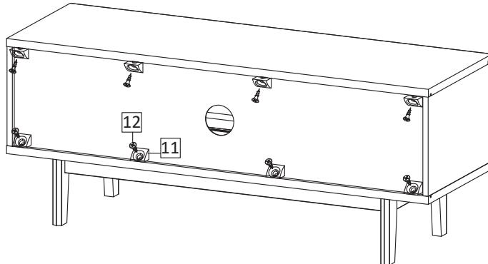
**STEP13:** Use Wedge (HW11), Screw M3.5x15.5mm (HW12) to tighten the back of media stand by using screwdriver. Please align the top board and bottom board in 90° position against the side board, before securing the wedges (HW11).
