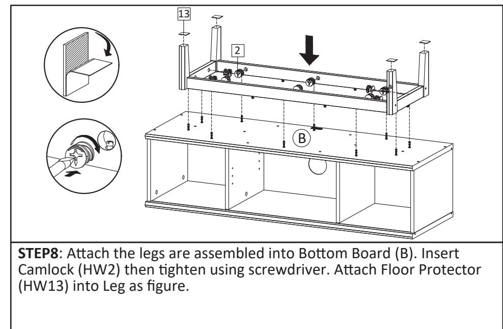
**STEP8:** Attach the legs are assembled into Bottom Board (B). Insert Camlock (HW2) then tighten using screwdriver. Attach Floor Protector (HW13) into Leg as figure.
