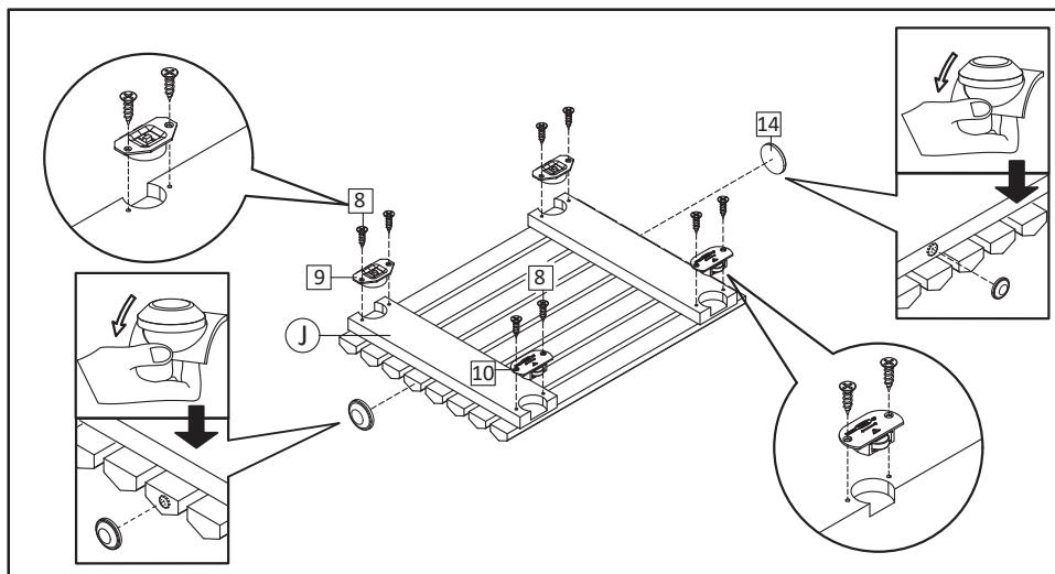
**STEP11:** The other Door frame will have 2 pcs of Bumper (HW14) , peel the back paper of it then attach on the Door . Please see different position of bumper on each side is needed. position as shown in the figure. Insert Sliding Top (HW9) and Sliding Bottom (HW10) using Screw M3.5x13mm (HW8) into Door (J).
