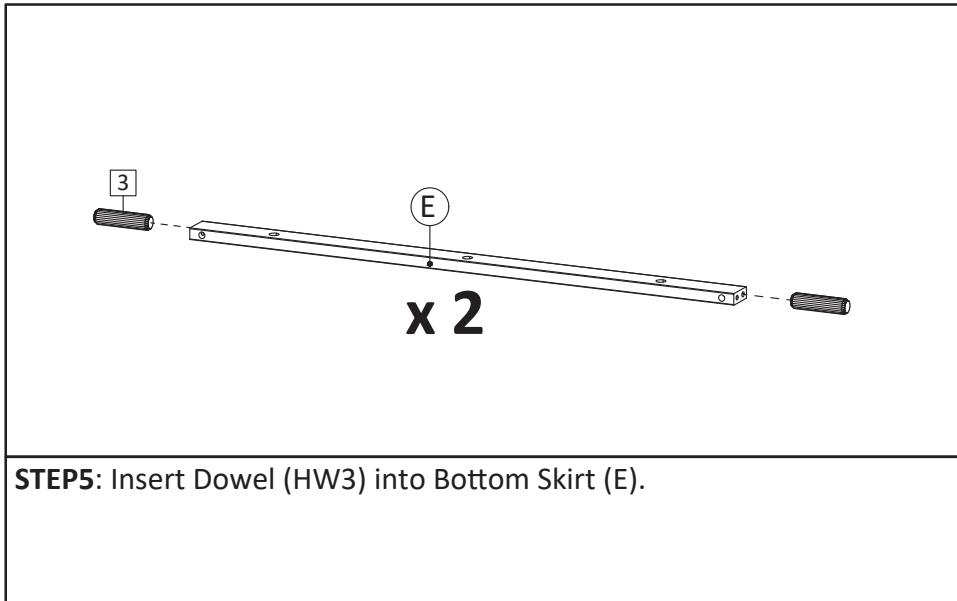
**STEP5:** Insert Dowel (HW3) into Bottom Skirt (E).
