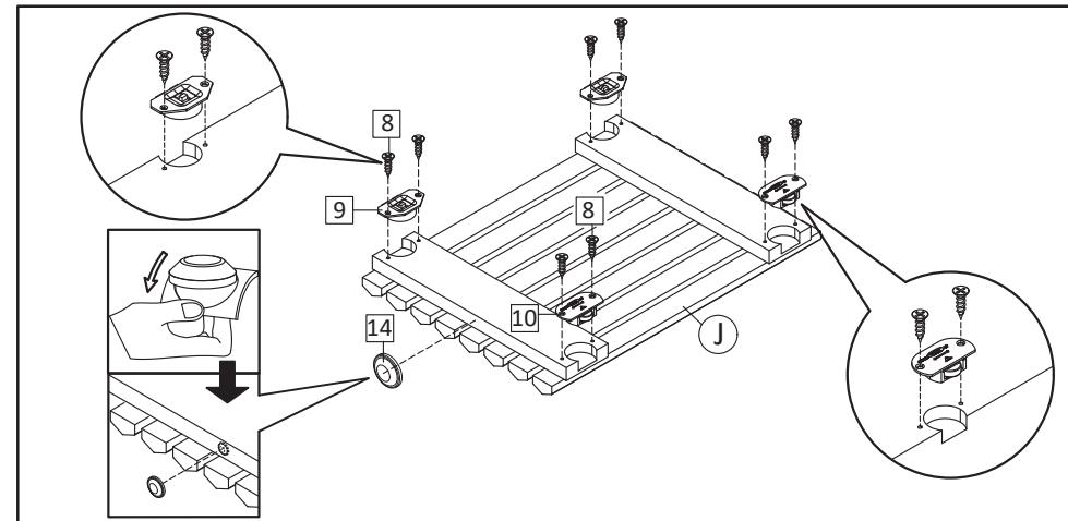
**STEP10:** Peel the back paper of Bumper (HW14) then attach on 1 of the Door with position as shown in the figure. Insert Sliding Top (HW9) and Sliding Bottom (HW10) using Screw M3.5x13mm (HW8) into Door (J).
