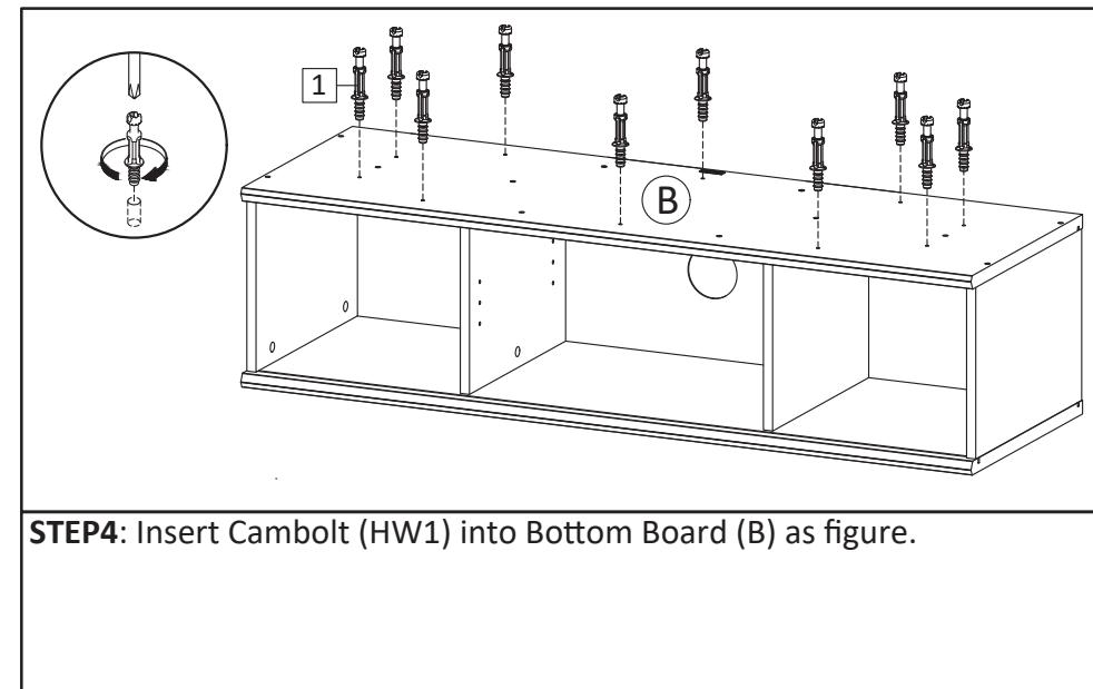
**STEP4:** Insert Cambolt (HW1) into Bottom Board (B) as figure.
