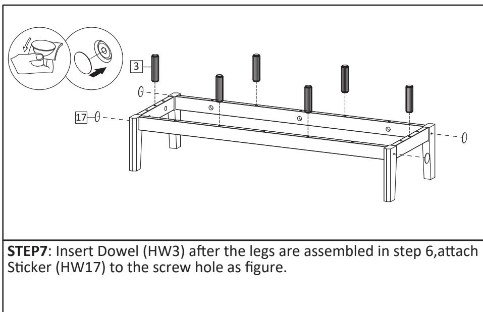
**STEP7:** Insert Dowel (HW3) after the legs are assembled in step 6, attach Sticker (HW17) to the screw hole as figure.
