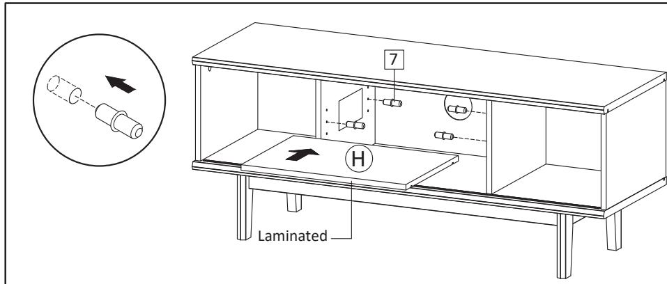
**STEP9:** Insert Shelf Pin (HW7) into the holes on Center Boards, on the desired level. Then place the Adjustable Shelf (H) by inserting the grooved line on the shelf into the shelf support.
