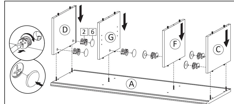
**STEP2:** Attach Side Boards (C&D) and Center Board (F&G), into Top Board (A) . Insert Camlock (HW2) then tighten using screwdriver. Put Screw Cap (HW6) over the camlock.
