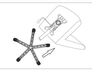
STEP 5: INSERT THE LEGS TO BAR LEVER. MAKE SURE THEY ARE IN CORRECT POSITION.
