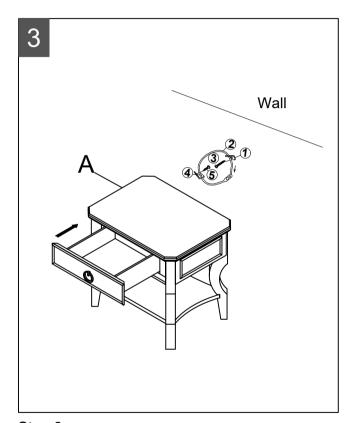
Step 3: Push the drawer close, Straighten up the assembled server. Following the installation instructions of anti-tipping to fix the server in the wall by 1 strap. assembly is completed.
