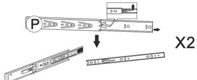
To extend metal sliders lift up the plastic lever.
