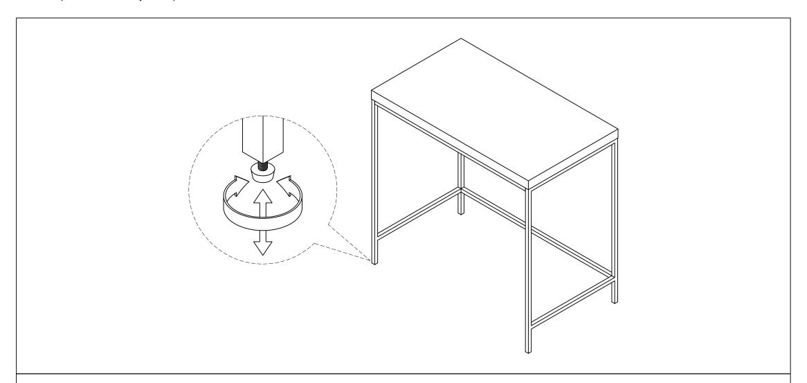
STEP 6 ADJUST THE ADJUSTER BOLT THAT HAS ALREADY ASSEMBLED TO THE LEGS TO STABILIZE YOUR UNIT
