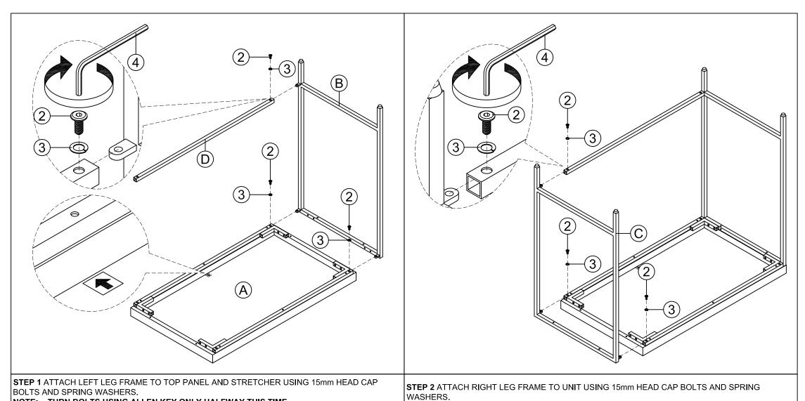
NOTE: - TURN BOLTS USING ALLEN KEY ONLY HALFWAY THIS TIME. - PAY ATTENTION TO THE POSITION OF THE ARROW LABEL IN THE TOP PANEL.
