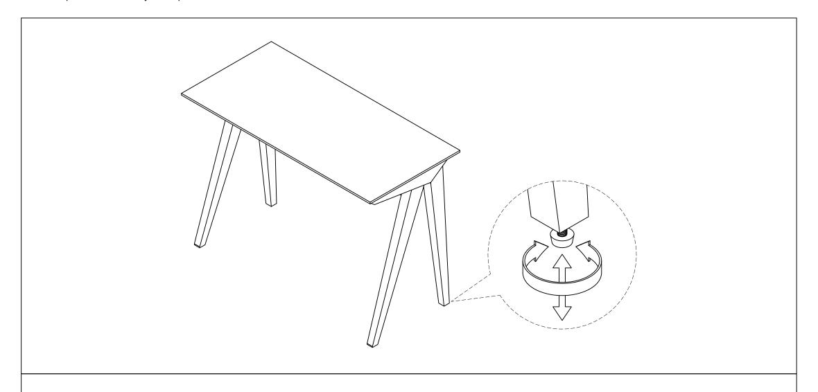
STEP 3 ADJUST THE ADJUSTER BOLT THAT HAS ALREADY ASSEMBLED TO THE LEGS TO STABILIZE YOUR UNIT
