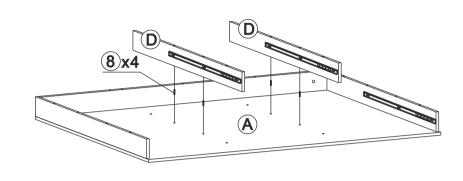
Insert HW® in part©, D, E, attach to part®, Use HW3 to install them together.
