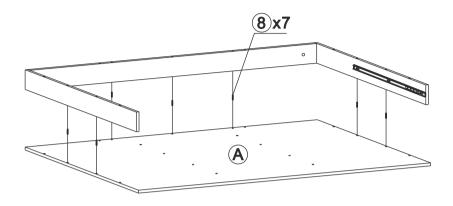
6 Insert HW® in part (A), install part (D) and (A) together.
