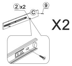
**3** Use HW2 to install the big piece of part P on both sides of part D.
