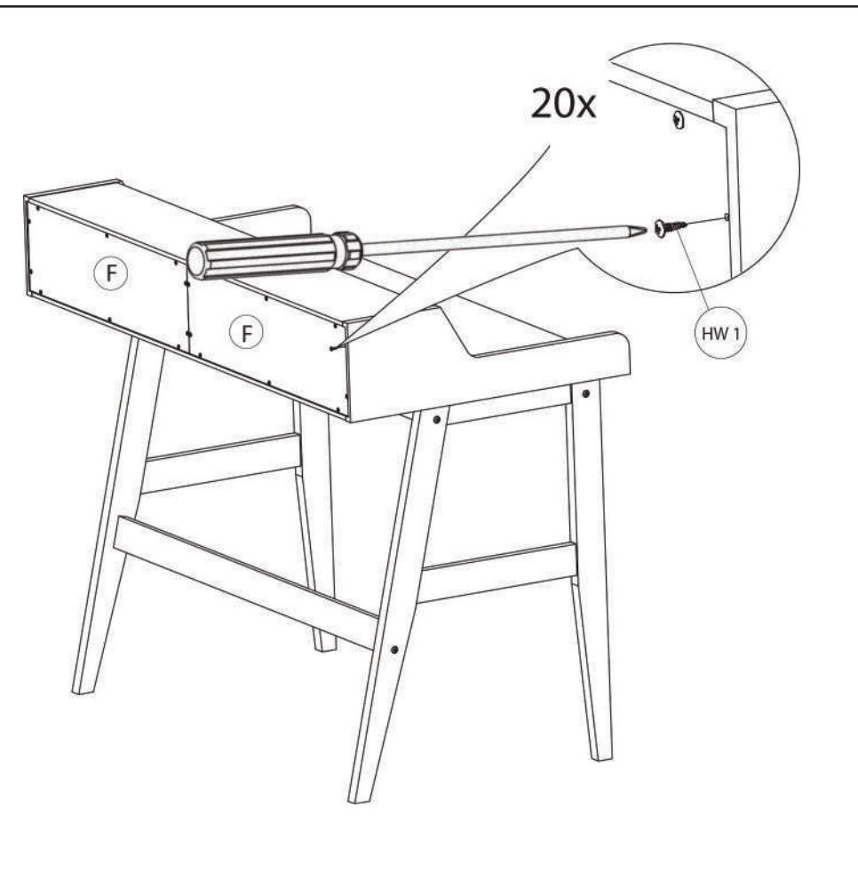
**Step 4 :** Place the back panel in position, then tighten all the screws.
