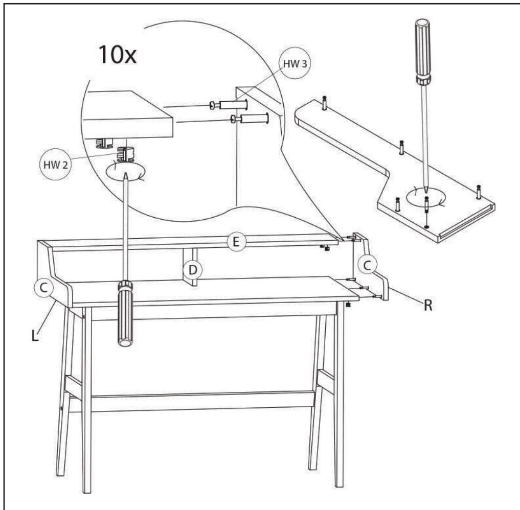
**Step 3 :** Attach all shaft (minifix) at both of the side panel, then assemble the parts.
