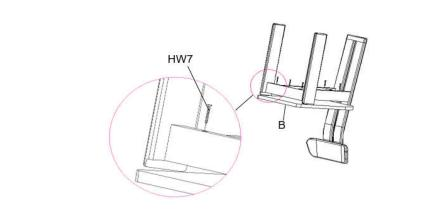
STEP 6: INSERT THE SEAT (B) AND CHAIR FRAME IN THE SCREWS BUT **DON'T** TIGHTEN COMPLETELY
