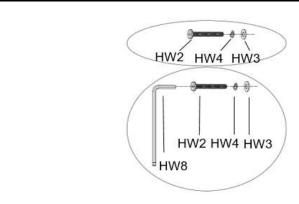
STEP 1: PUT THE WASHERS ON THE BOLT IN THE ORDER SHOWN IN THE PICTURE
