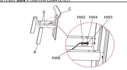
STEP4: INSERT THE BACK LEGS © AND THE FRONT LEG FRAME (A) IN THE BOLTS BUT **DON'T** TIGHTEN COMPLETELY
