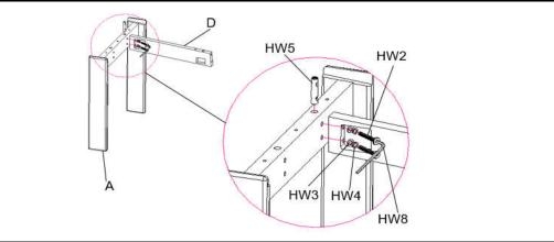
STEP 2: INSERT THE FRONT LEGS FRAME (A) AND THE FIRST SIDE STRETCHER (D) IN THE BOLTS BUT **DON'T** TIGHTEN COMPLETELY
