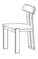
STEP 7: PUT THE CHAIR UPRIGHT AND MAKE SURE ALL LEGS ARE LEVEL, THEN FIRMLY TIGHTEN BOLTS WITH ALLEN KEY WHILE THE CHAIR IS UPRIGHT AS PICTURED ABOVE
