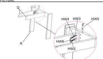
STEP 3: INSERT THE FRONT LEGS FRAME (A) AND THE SECOND SIDE STRETCHER (D) IN THE BOLTS BUT **DON'T** TIGHTEN COMPLETELY
