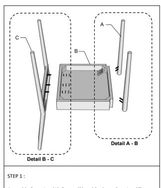
Assemble Front Leg (A), Seater (B) and Backrest-Rear Leg (C)
