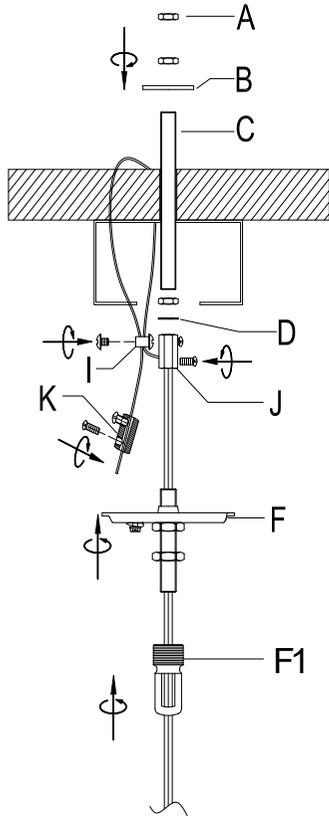
**Step 3:** Raise the threaded rod (C) thread to the cluster (J), then attach to the ceiling, secure with metal washer (B) and hex nut (A). Wrap the steel wire rope around the beam and lock it with the steel cable buckle (I) and (K). Tighten Mounting bracket (F) to Cluster (J), then fix Canopy Loop (F1) to Mounting bracket (F).
