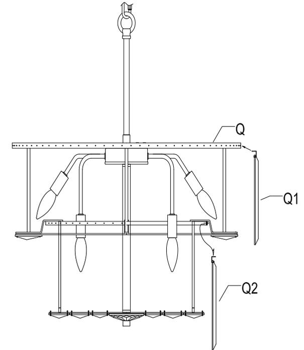
**Step 8:** Install the crystal (Q1)(Q2) to the groove or fixture body (Q),
