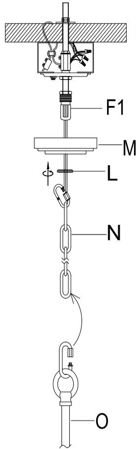
**Step 6:** Attach the canopy (M) to the ceiling with Canopy ring (L), Attach two ends of Chain (N) to Canopy Loop (F1) and Center rod (O).
