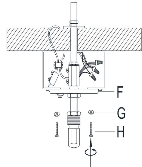
**Step 5:** Install the mounting bracket (F) to the junction box with plain washer (G) and outlet box screw (H)
