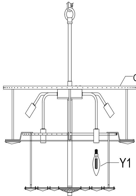
**Step 7:** Install the light bulb (Y1) to the socket.
