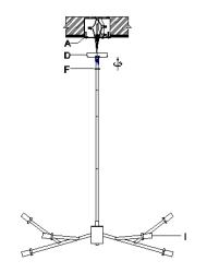
**Step 4:** rotate and install the lamp body (I) clockwise to the mounting plate (a). Fix the canopy (d) on the junction box, and rotate the canopy nut (f) clockwise to fix it.
