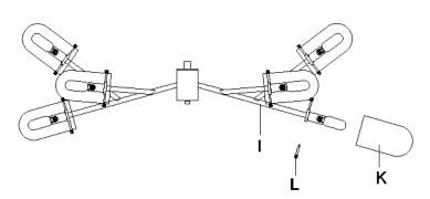
**Step 6:** Place the crystal (k) on the lamp body (I), and then tighten he Coronet Screw (L) on the lamp body (I).
