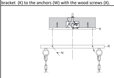
Step 5: Fix the canopy (R) on the mounting bracket (K) with the Screw (N).
