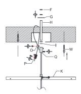
**Step 2:** Determine the position for the mounting bracket (K) and mark the four location holes. Drill a 1/4 in. hole at each marked position, and insert an anchor (W) into each hole. Pass wire and cable through Mounting bracket (K) and out from side hole of Cluster (Q). Wrap the steel wire rope around the beam and lock it with the steel cable buckle(O) and (P).
