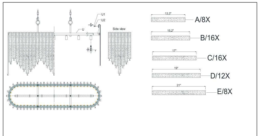
**Step 6:** Install the light bulb (V) to the socket. Take off the parts (U1) from Fixture body (U), Pass through Glass strip (A), (B), (C), (D), (E) and fix to fixture body. While locking the glass please have glass be vertical and don't lock too tight to avoid the glass be slant.
