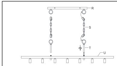
**Step 1:** Tighten Center rod(T) to Fixture body(U). Pass wire and cable through Chain(S) and Canopy(R), Fix two ends of Chain(S) to Center rod(T) and Canopy(R).
