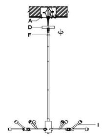
**Step 4:** Rotate and install the lamp body (I) clockwise to the mounting plate (a). Fix the canopy (d) on the junction box, and rotate the canopy nut (f) clockwise to fix it.
