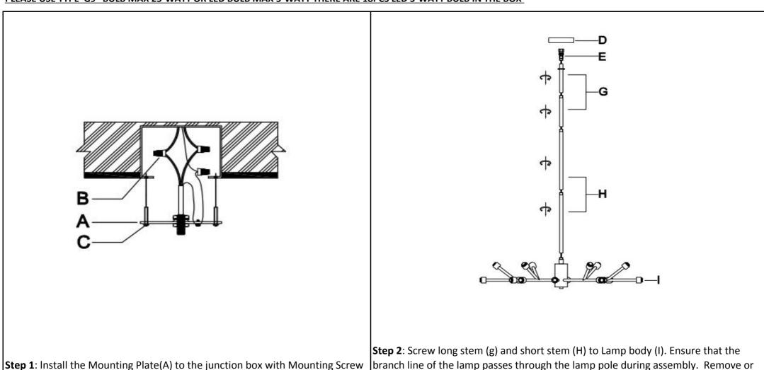
add stems to adjust height. Then screw the lifting ring (E) onto the valve stem.
