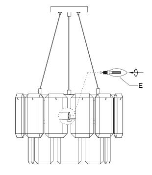
**Step 6:** Install the light bulb (E) to the socket.
