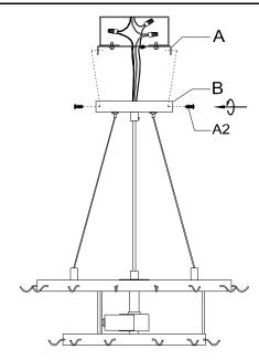
**Step 4:** Attach the canopy (B) to the mounting bar (A), secure with canopy screw (A2).
