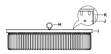
**Step 6**:Insert the light bulb (J) into the lamp Sockets. Insert the crystal bar (K) on the lamp body (I).
