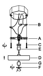
**Step 4:** Install the Mounting Plate(A) to the junction box with Mounting Screw(C). Seperate the Mounting Plate(A) from the Canopy(D) by turning the Canopy Nut(F) anti-clockwise.
