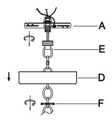
**Step 5:** Attach the Canopy(D) to the junction box and fix it by turning the Canopy Nut(F) clockwise.
