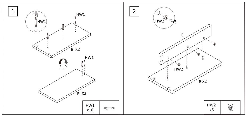
STEP1: Insert 10x cam bolts (HW1) into panel [B]. Tighten with a screwdriver.
