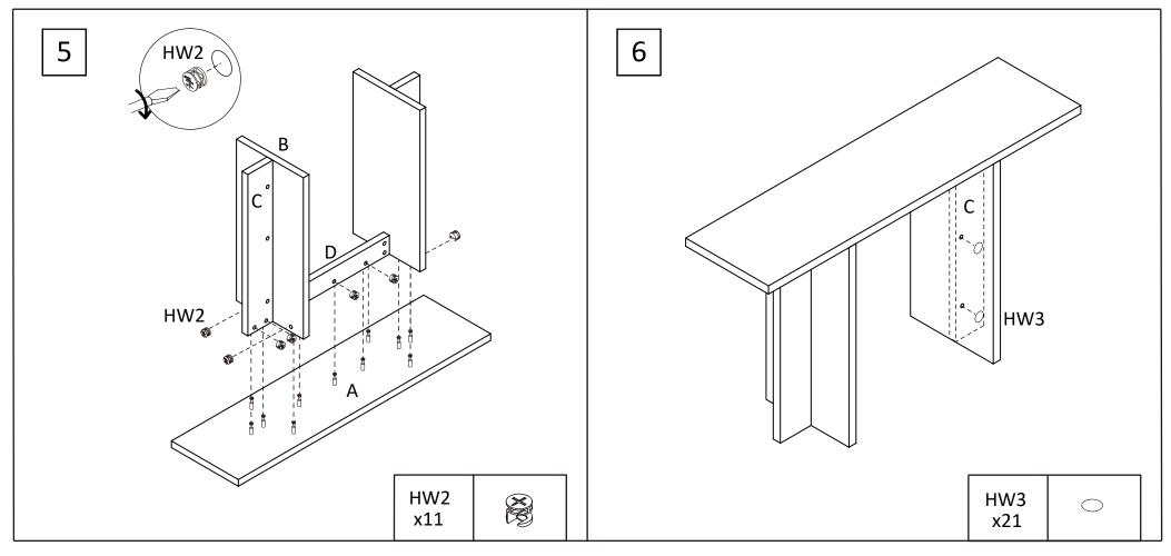
STEP5: Attach panels [B], [C] and [D] to panel [A] secure with 11x cam lock (HW2). Tighten with a screwdriver. STEP6: Attach 21x stickers (HW3) to panels [B], [C] and [D]. You're done, enjoy!
