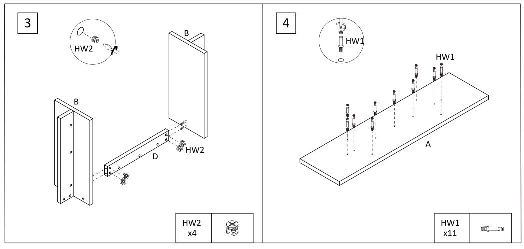
STEP3: Attach panels [B] to panel [D] secure with 4x cam lock (HW2). Tighten with a screwdriver.
