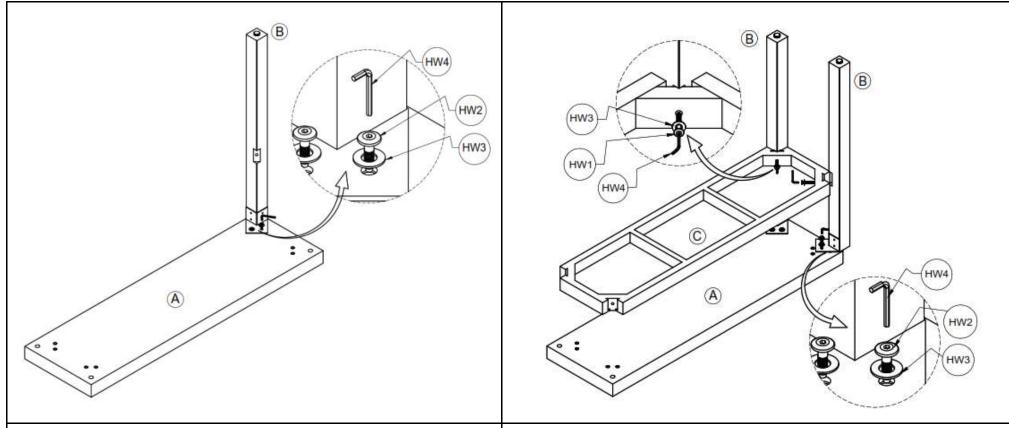
**STEP 1:** Place the top panel (A) upside down then attach the legs (C) by inserting the Bolts (HW1) and Flat washer (HW3) then tighten with the Hex key (HW4).
