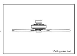
Standard drop ball installation is suitable for general building installation, ramp drop ball installation is suitable for installation on the inclined plane (inverted as inclined roof). The ceiling type installation is suitable for the lower floor space.
