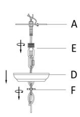
**Step 4:** Install the Mounting Plate(A) to the junction box with Mounting Screw (B). Seperate the Mounting Plate(I) from the Canopy(H) by turning the Canopy Nut(F) anti-clockwise.
