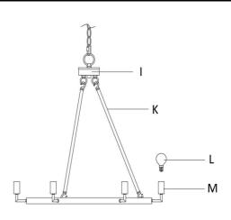
Step 6: Insert the bulbs (L) into the Sockets
