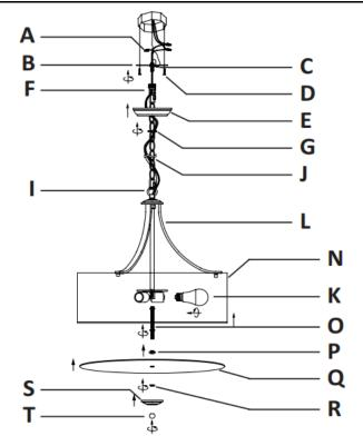
**Step 5:** Attach the Mounting Plate (B) onto the junction box with two Mounting Screws (D).
