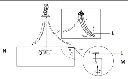
Step 3: Adjust the angle of the spider of the Lamp Body (L).
