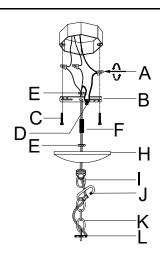
**Step 1:** Unpack all parts from carton carefully.Place the Canopy (H) onto the Hanging Loop (I)Screw the Nipple (F) into the threaded portion of the Hanging Loop (I) and fix it by turning the Canopy Nut (F) clockwise till tight.Attach the Closable Link (J) onto the Hanging Loop (I).
