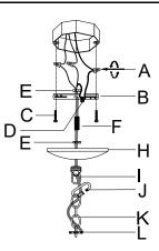
**Step 4:**Separate the Crossbar (B) from the Canopy (H) by unscrewing the Canopy Nut (L).
