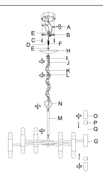
Step 5: Install the Crossbar (B) to the junction box with Outlet Box Screws (C). Attach the Canopy (H) to the junction box and fix it by turning the Canopy Nut (L) clockwise. Slide the Tubes (P) over the sockets, Insert the G9 bulbs(Q) into the sockets, and then thread the Bulb Shields(O) to the Fixture Body (R) as shown.
