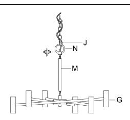
**Step 2:** Thread the Stem (M) to top of the Fixture Body (Q),and then thread the Fixture Loop (N) to the Stem(M).Attach the Closable Link (J) onto the Fixture Loop(N).
