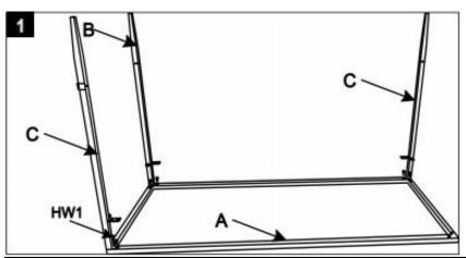
**STEP 1**: Attach Legs (B&C) and Top (A) together using Allen bolts(HW1).
