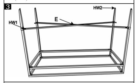
**STEP 3**: Attach Legs (B&C) and Shelf (E) together using Allen bolts(HW1). Tighten all the Allen Bolts.
