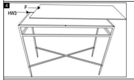
**STEP 4:** Place the Glass Mats (HW3) on to the frame. Then place the Glass (F) onto the Top (A).
