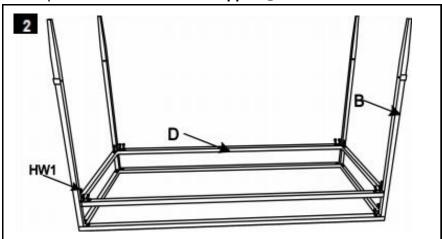
STEP 2: Attach Legs (B&C) and Shelf (D) together using Allen bolts (HW1). Do not fully tighten.
