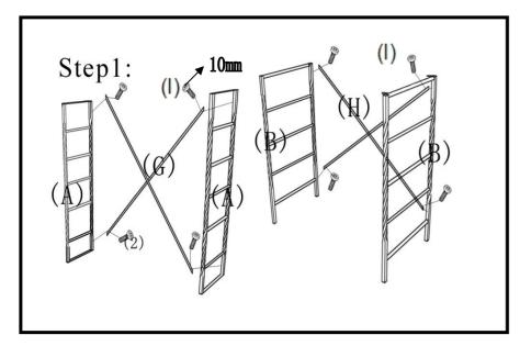
**Step 1**Attach the bars (G) (H) to the side stands(A) and the legs (B), use allen key to tighten the bolts(I)
