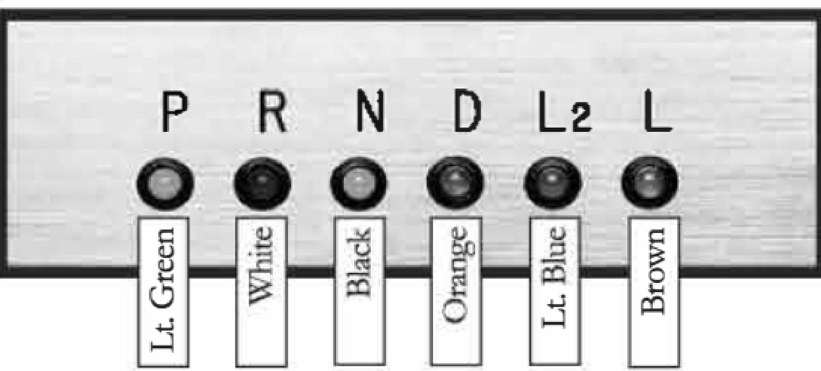
Connect the red wires from each indicator light in the following order: Park to Lt. Green wire, Reverse to White wire, Neutral to Black wire, Drive to Orange wire, Second to Lt. Blue wire, Low to Brown wire. The Ground for the indicator lights is done by tying all the yellow (or black) wires together and running them to a good ground.
