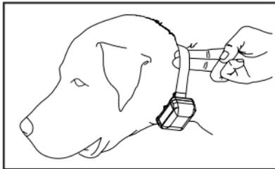
A proper fit is necessary for the iQ No Bark Collar to work optimally. Both contact points must be in contact with your dog's skin at all times for a consistent stimulation. A loose fitting collar can cause the contact points to rub against the skin and cause irritation.
