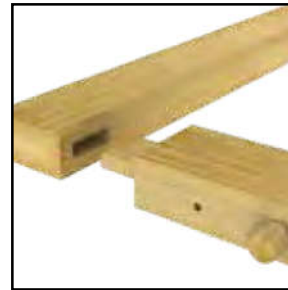
Mortise & Tenon Joint Frame
