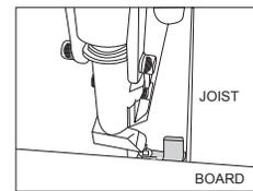
With the magazine still resting on the joist, slide the nose of the gun to the right removing it from the attached fastener.
