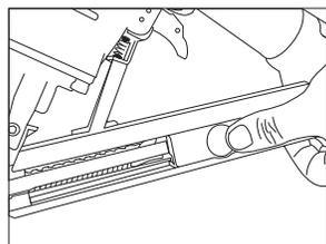
Pull back the spring coil until it locks onto the back of the sleeve.
