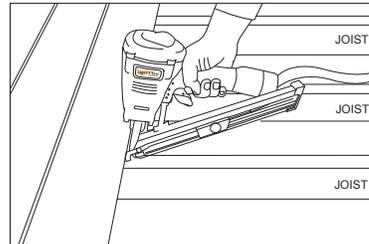
Holding the gun upright, insert the horned tab into the groove of the deck board directly over the support joist.
