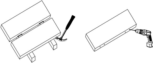
When not starting against the house or when very dense composite materials are used, bouncing may occur during installation of first few boards. Following these steps can ease the installation of the first 3-4 courses if difficulties arise.
