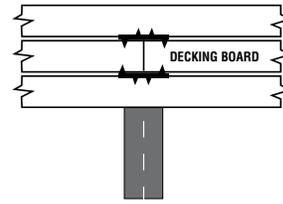
When butt jointing deck boards, drive the first deck board onto prong with the seam end centered over a support. When installing the second deck board, start installation at the butt seam if you prefer a small gap in the butt seam. If you prefer no gap in the butt seam, start installation at the outside end of deck board and work toward seam.
