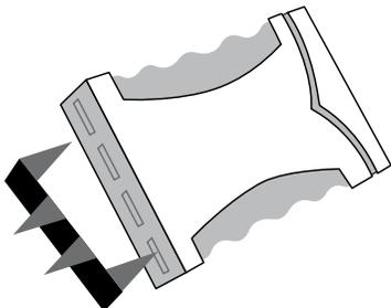
Insert prongs of fastener into slots in installation block.
