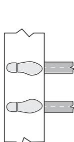
**a** To ensure even deck surface, make sure you are standing on deck board when installing with block.
