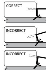
**e** Check position of prongs – make sure prongs are straight out.
