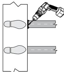
**d** Install screw at a 45° angle, through center hole of fastener and down into support joist.
