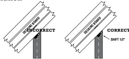
Where deck is in walled corner of house, always start with small triangular piece of decking in that corner and work your way out. When working with small pieces, it is advisable to mark prong impressions and predrill. When installing Tiger Claws, offset the center 3/4" towards the long point of joist, so screw will not exit side of joist when driven.
