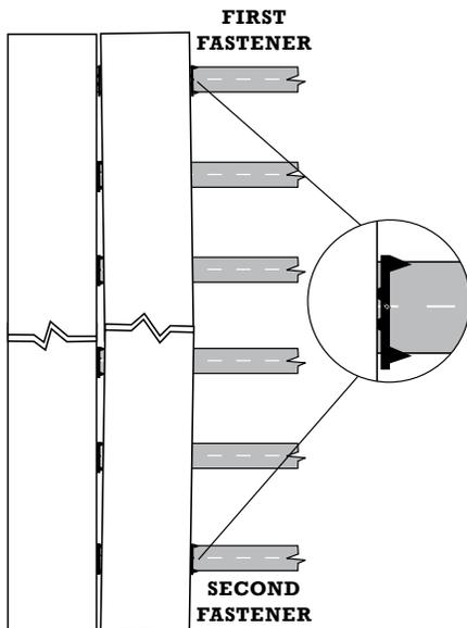
Once the end of the board is reached, drive end until proper gap is achieved, then install Tiger Claw fastener & screw to hold in place like at the beginning of board.
