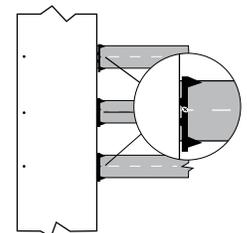
**f** Install one (1) Tiger Claw fastener and screw into edge of deck board at each support joist. Your deck surface should look like this before proceeding with the next section.
