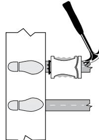
**b** Place block over joist & strike with hammer, then screw into joist.
