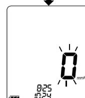
3. When inflation is complete, deflation starts automatically and ♥ (heart mark) blinks, indicating that the measurement is in progress. Once the pulse is detected, the mark blinks with each pulse beat.
