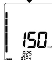
4. When the measurement is complete, the systolic and diastolic pressure readings and pulse rate are displayed. The device announces the measurement results. The cuff exhausts the remaining air and deflates completely.
