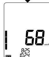
Note: If an appropriate pressure is not obtained, the device starts to inflate again automatically. To avoid re-inflation, see “Measurement with the SET Pressure” on the next page.
