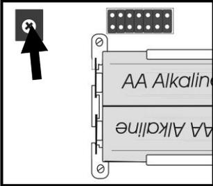
To adjust audio volume, first remove the front plate as described in the previous, “Low Batteries” section. In the upper left corner of the front plate’s circuit board, you’ll find a quarter of an inch square plastic cube with a small Phillips head screw in the middle of it. To increase volume, turn the screw clockwise with a small Phillips head screwdriver. To decrease volume, turn counterclockwise.
