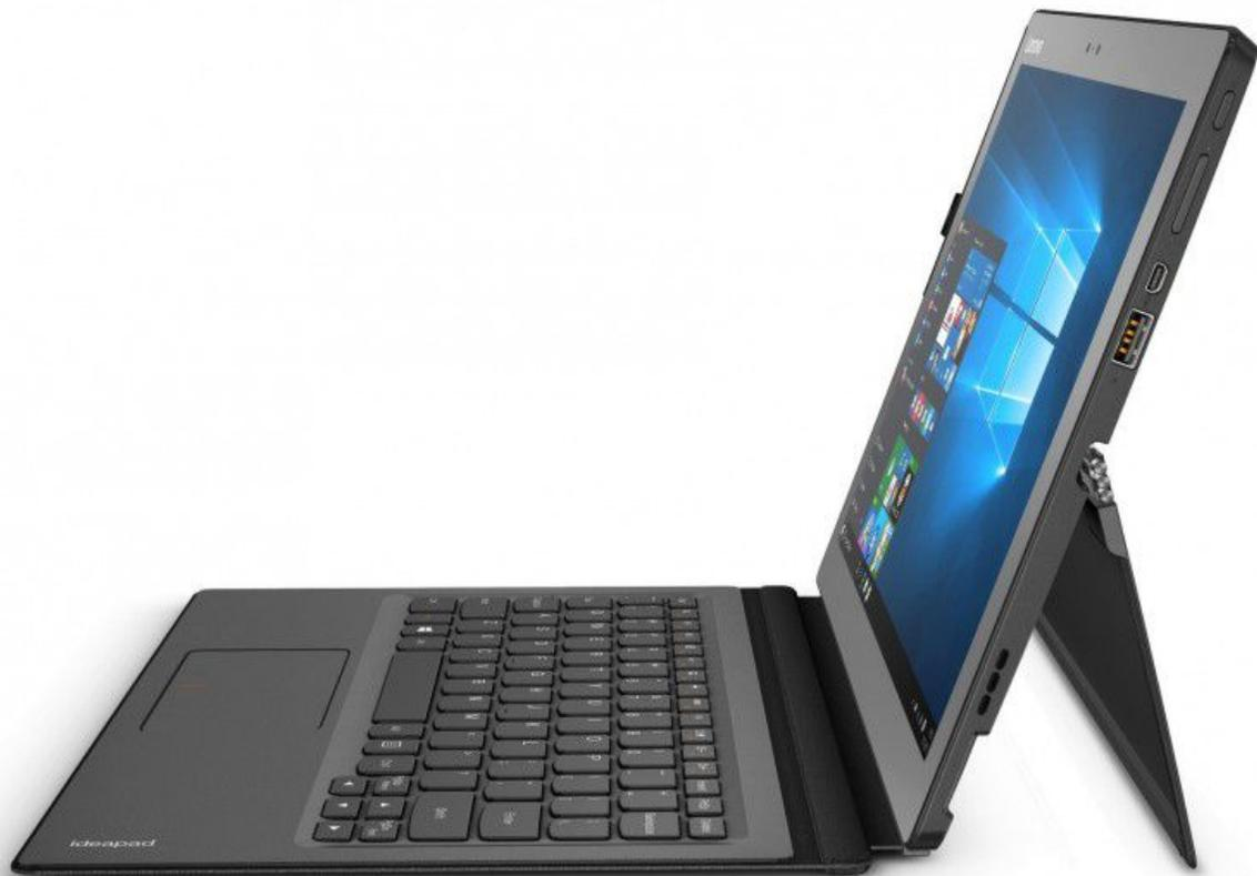
While inserting the tablet back onto the stand, ensure that the power button is on the bottom left. If it's on the top right it means the tablet has been inserted upside down and the tablet camera will not line up with the respective camera hole on the stand.
