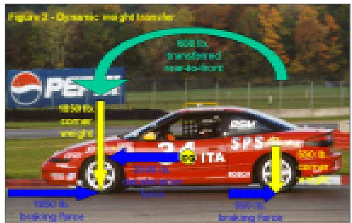
In Figure 3 (the beginning of what we call a “fishbone diagram”—more on this later), we see how our 2500 pound vehicle with 50/50 weight distribution at rest transfers weight based upon deceleration. Under 1.0g of deceleration (and using some typical values for our vehicle geometry) we have removed 600 pounds from the rear axle and added it to the front axle. That means we have transferred almost 50% of the vehicle’s initial rear axle weight to the front axle!
