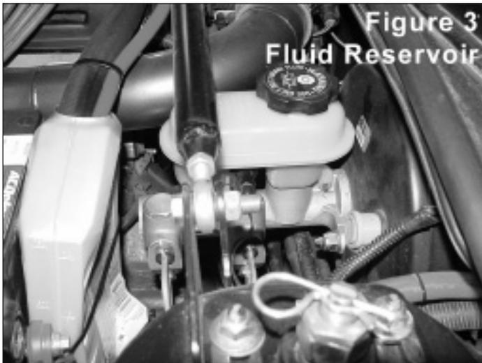
As brake fluid ages it absorbs water. Unfortunately, when the water get sucked up, it lowers the boiling point of the fluid, and it doesn't take too long until the resulting mixture has a boiling point much lower than when it was new.
