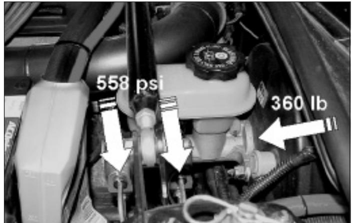
Figure 2 – The master cylinder generating pressure
