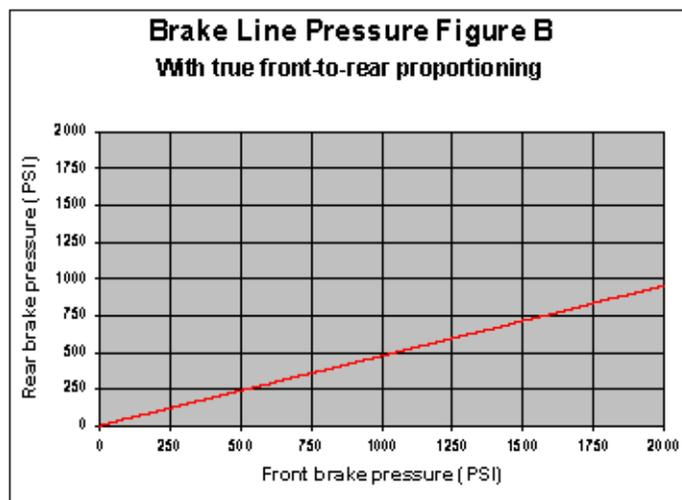
Because of the complexity involved with a dual-master cylinder set-up, this type of proportioning is rarely—if ever—found on passenger cars, and certainly not on modern trucks.
