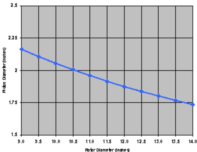
Unfortunately, too many junkyard swaps do not take this factor into account, and those poor trucks end up with both bigger rotors and larger pistons, which serve to drastically shift the bias even more forward. While rock-solid stable under braking, stopping distances will go *up* dramatically.
