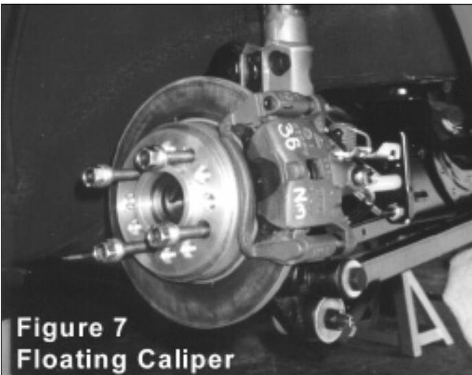
While the fixed type caliper is more efficient in general, floating calipers typically take up less space and are cheaper to manufacture. For this reason, almost every large-volume production truck and car on the road today (including your Ram) utilizes floating calipers.
