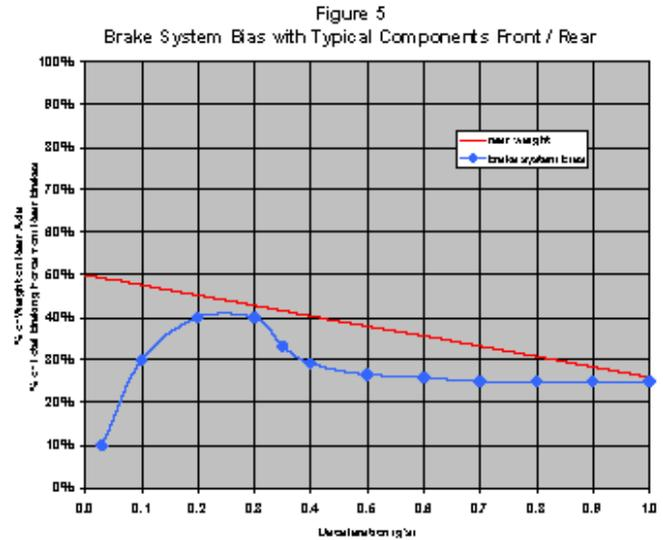
And here’s a free tip—effects of compromised brake bias on the street not only include sub-optimal stopping distances, but also include sub-optimal brake pad life. If a truck is too heavily front-biased in the deceleration range it typically operates in, it will wear front pads more quickly due to the fact that the rear brakes aren’t doing as much of the stopping work as they could be. However, the rear brake pads will probably last forever . . . sounds familiar, doesn’t it?
