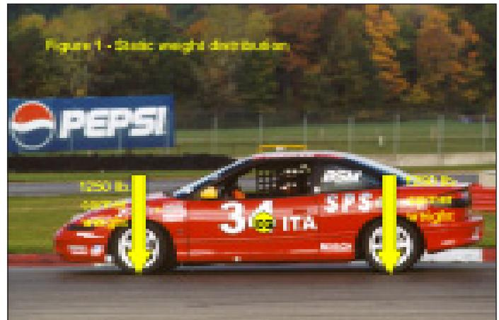
Note that when at rest, there are no horizontal (left or right) forces acting on the vehicle. All of the forces are acting in a vertical (up and down) direction. But what happens to the vehicle when we start to apply forces at the tire contact patch to try to stop it? Let's find out.
