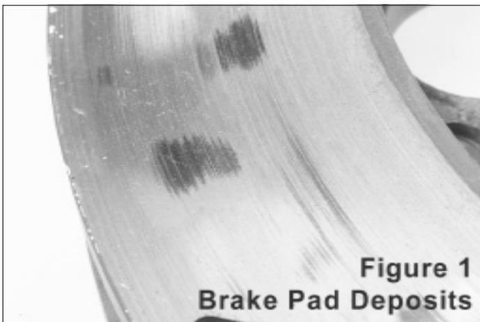
TV can also be generated through overheating of the rotor. When the rotor gets really, really warm, it will actually develop isolated spots which are hotter than the surrounding material. These hot spots will also accelerate wear locally, creating a thick and thin pattern on the rotor face. Again, this will only get worse with time until the TV is felt by the driver and his (or her, as the case may be) passengers.
