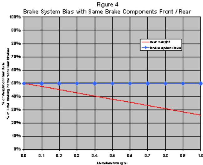
Evaluating this chart, we see that the vehicle will always be rear-biased. That is, the rear brakes will always be applying more force at the tire contact patch than the weight of the rear axle can sustain. This vehicle will always lock the rear brakes before the front. Not so good.
