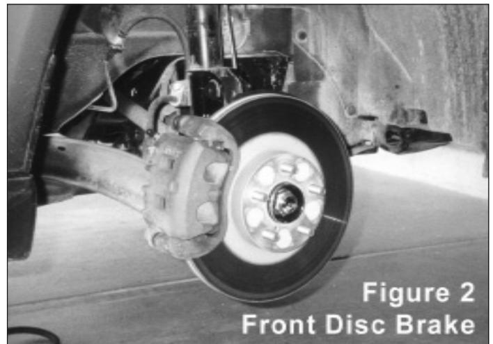
Disc brake calipers employ a square sectioned piston seal to pull the caliper piston back into its bore when the brake pedal is released. However, the seals are designed so that they don't pull the pistons back quite so far that the brake pedal feels mushy when you need it the next time. This compromise in design leads to brakes that do exhibit a small amount of drag when released, but minimal pedal dead travel when applied.
