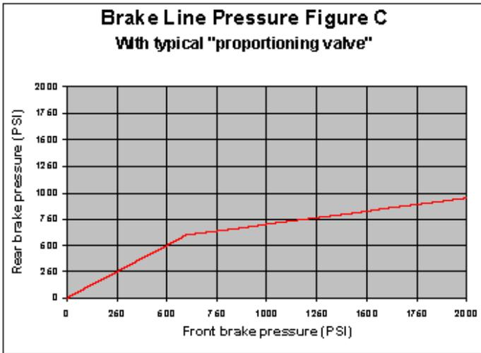
Because of their compact size and relatively low cost, these devices can be found on nearly every vehicle requiring rear brake pressure reduction to achieve optimum brake bias. Pickup trucks fall neatly into this category.
