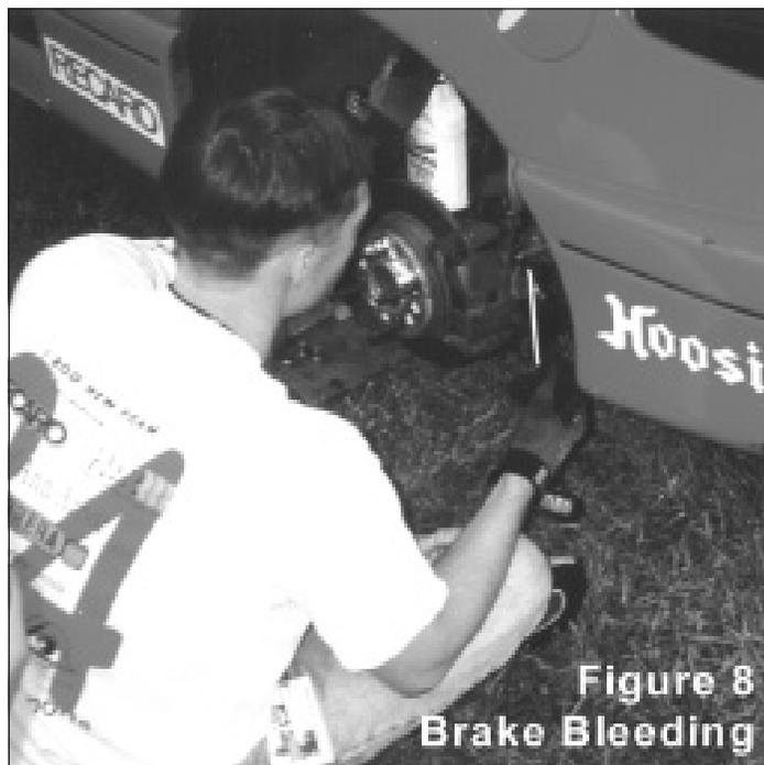
15. When all four corners have been bled, spray the bleeder screw (and any other parts that were moistened with spilled or dripped brake fluid) with brake cleaner and wipe dry with a clean rag. (Leaving the area clean and dry will make it easier to spot leaks through visual inspection later!) Try to avoid spraying the brake cleaner directly on any parts made of rubber or plastic, as the cleaner can make these parts brittle after repeated exposure.
