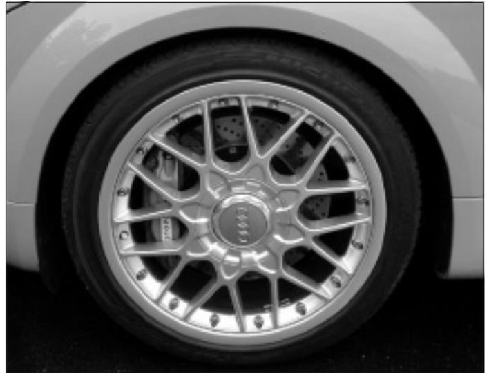
Figure 7 – Filling the wheel with brake hardware
