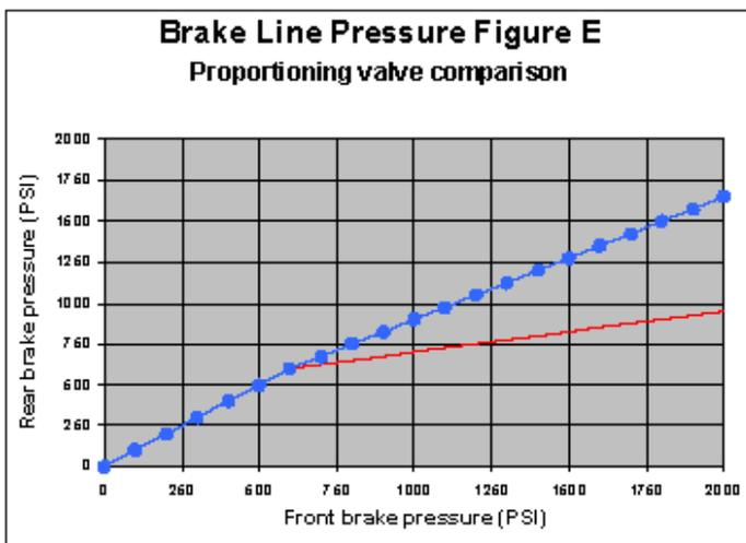
So how does one select the right kneepoint and slope? Without the test and measurement resources of a major automotive manufacturer, it's next to impossible to say. Of course, you could trial-and-error your way into a situation that you believe to be appropriate, but without testing under all conditions of loading, speed, and road conditions there might be one rear-biased operating condition just waiting to bite you.
