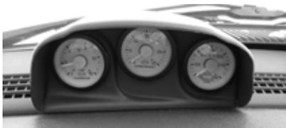
As mentioned, with a gauge installed you can use the boost readings as a diagnostic check of the engine's performance. The engine will need to see a full throttle, loaded condition in order to make its maximum boost number. The easiest way to do this is to drive the truck up a hill. No hills in Kansas? Apply the brakes to load the engine.
