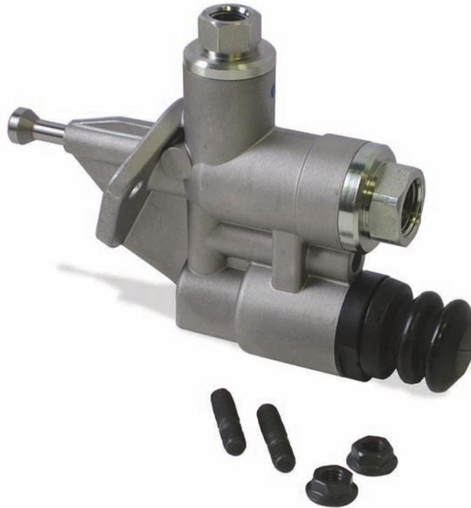
Here is the secret: When you remove the fuel lift pump, install the longer mounting studs that we are sending to you in this kit. These studs allow you to slip the new pump, heater and gaskets easily into place. Tighten the nuts to 18 ft. lbs. of torque.
