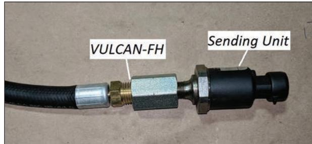
This is a picture of the opposite end when using a mechanical gauge:
