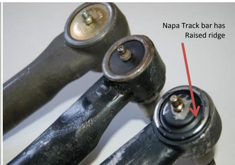
**Moog:** This kit will not work on this bar. This is a 2" diameter bar. Stop and call us for our Exchange program.
