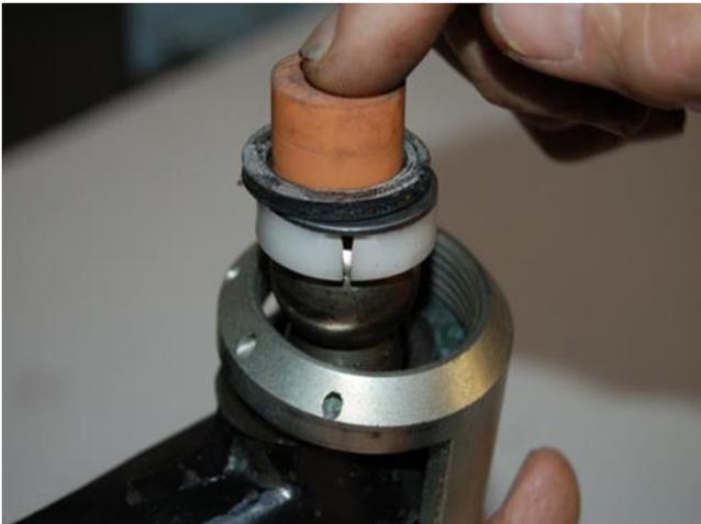
**Step 9:** Now install the threaded nut and tighten by hand until it won't go further. Then tighten with 1/2 inch drive ratchet until tight. You will feel it bottom out. This is generally about 35lbs of torque.
