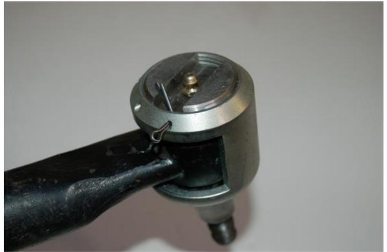
Adjusting A Luke's Link Track bar kit. Luke's Link comes with 3 small metal washers. These are used for adjusting the Luke's Link in case steering gets a little loose (wonder). To adjust, leave truck on ground with steering wheel unlocked, remove cotter pin and unscrew plug. Put one spacer under spring. Replace plug and cotter pin. This will take up the play in the end.
