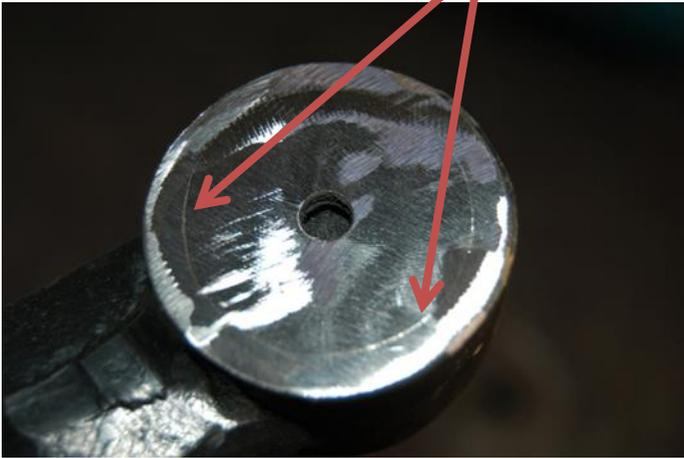
**Step 5:** Break loose encasing seal. With bar in vice as show, hit with hammer to break loose. Usually 2 or 3 hits will break loose. Remove parts from inside bar and throw away. There is metal Race under ball stud, if it falls out, please put back in. Do not damage ball stud. It must be reused.
