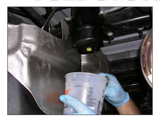
Now, with the canister, fuel filter and diesel fuel baggie or bucket removed, let's take a look at the yellow (lack of drain) drain plug. Because it has a "T" shaped head, the plug doesn't drop out of the canister. When it is unscrewed it just doesn't have the right cuts in the plastic to allow fuel to drain.
