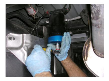
In the trucks we've worked on we've determined that the removal of the canister would not result in a diesel fuel bath IF we could get the fuel to drain from the yellow plastic drain valve. However, the drain valve doesn't drain.
