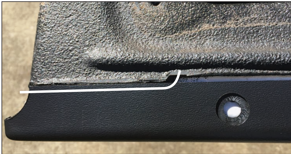
See how the cover does not fit flush due to the excess spray in the bed liner (at the left corner). The tailgate protector will have to be trimmed to fit (follow the white line).
