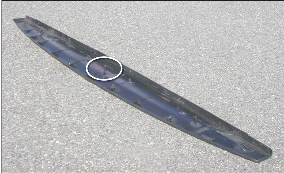
This is the underside of the OEM tailgate cover. Notice only one tab remains unbroken.
