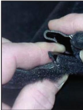
This photo shows the J-Clip that attaches the seat-back cover together as it is unhooked.
