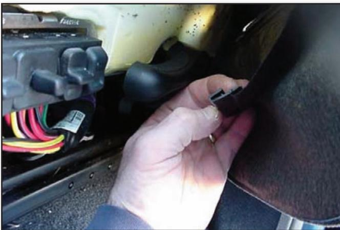
In removing the J-Clips, it helps to put on a pair of rubber gloves to protect your hands. Should your hands slip, the gloves will keep your hands from being cut on sharp metal brackets under the seat.
