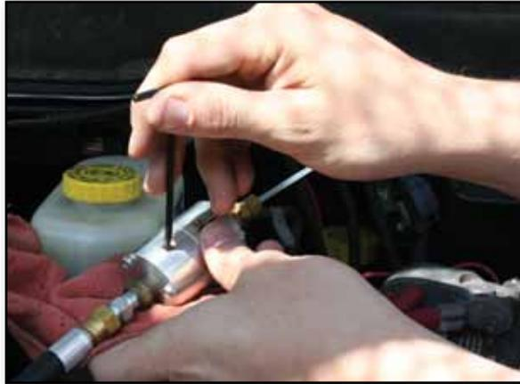
5. Next, connect the fuel supply hose to the isolator, cycle the lift pump and bleed the air out of the hose by loosening the bleed screw.
