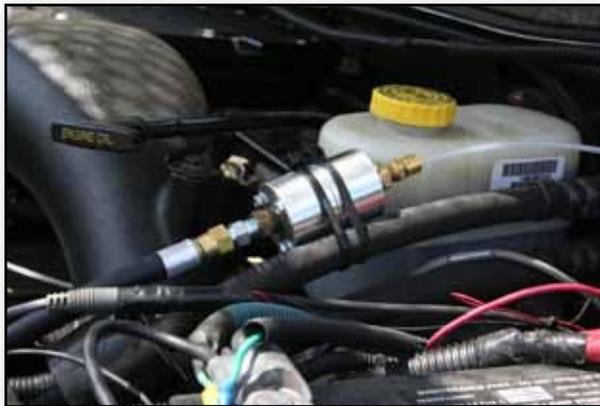
6. Here is an example of a convenient location for mounting the isolator.
