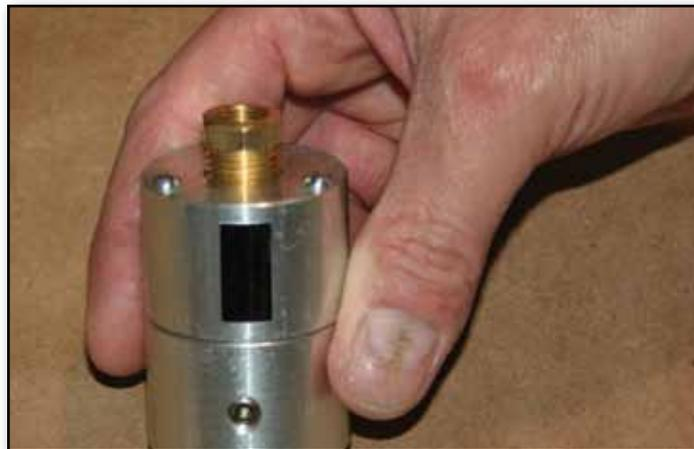
3. Fill this side of the isolator with coolant and insert a fitting into the gauge side of the isolater. Hand tighten for now.
