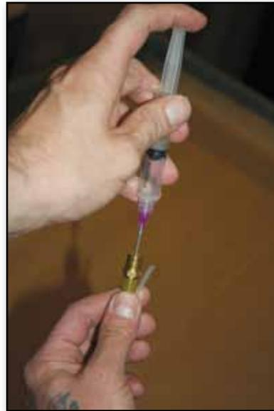
5. Leave 1 to 2 inches of air in the line to allow for coolant expansion. Tighten the fitting at the isolator to keep the coolant from leaking.
