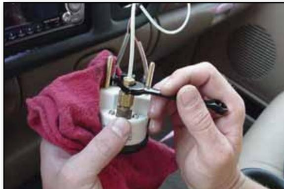
4. Attach the line to the back of the gauge and tighten the fitting. Take care not to damage the gauge.
