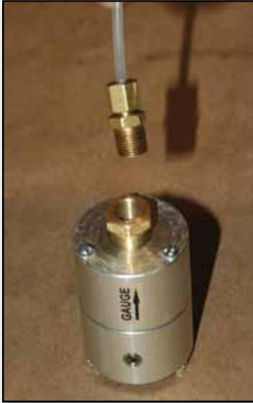
4. Fill the plastic tube with coolant. It's best to expel as much air as possible. To accomplish this, loosely attach the plastic line to the isolator using the supplied fittings and then use the supplied syringe to fill the plastic line.
