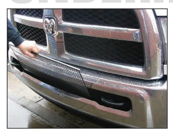
Installing the Intercooler Guard is simply a matter of putting it through the bumper opening and attaching it to the intercooler. Once you have the Intercooler Guard inside the bodywork, you can get started.
