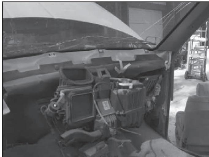
**Another view of the HVAC box with the dashboard assembly removed.
