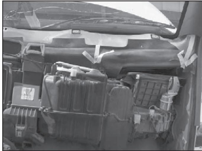
**View of the HVAC box with the dashboard assembly removed.
