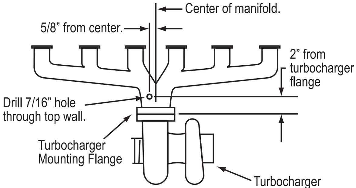
Locate a point two inches from the turbo mounting flange centered on the exhaust manifold, then move forward or rearward on the manifold 5/8," then center punch for drilling. If you are using a 1/4 NPT probe, drill a 7/16" diameter hole straight down through one wall. If you have a 1/8 NPT probe, drill a 5/16" diameter hole. Putting axle grease on the drill and tap will help prevent shavings from falling into the manifold. Tap threads using 1/4 NPT pipe tap or the 1/8 NPT pipe tap.
