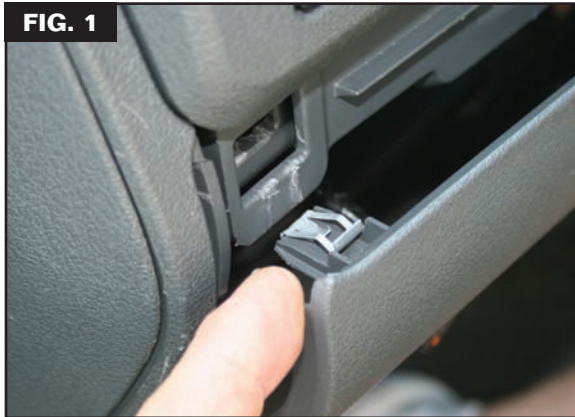
Drop the knee bolster panel by grabbing under the steering column and pulling out and down. As you can see, the top of the bolster is held in place with expansion clips.
