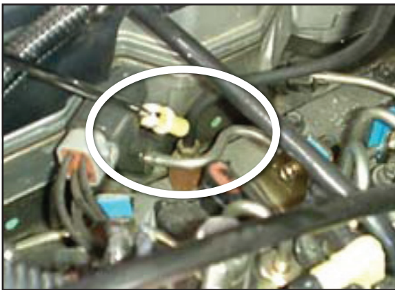
The pointer shows the boost bolt and boost line installed in a 5.9-liter engine.
