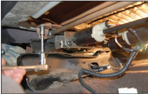
'94-'02 Truck: Removing the seat bottom frame.
