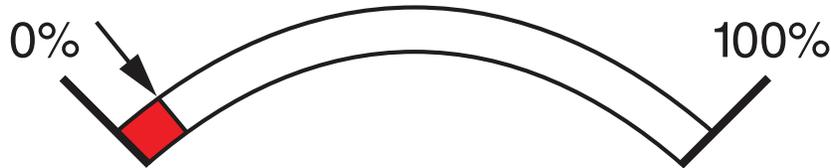
This aftermarket replacement sensor is designed a bit differently only in the "IDLE" portion of it. Look at the drawing above and take notice to the shaded area. The first few degrees of movement in the beginning is the "IDLE VOLTAGE". The voltage stays constant (does not rise). The end of the shaded area is the point at which voltage rises, thus engine RPMs increase.
