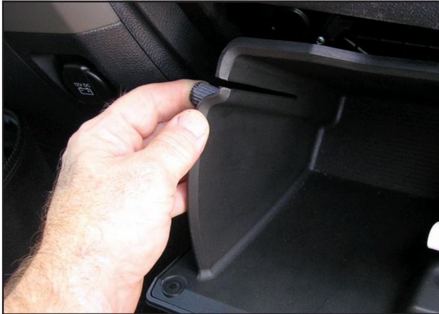
Pinch in both the V-sides, drop the glovebox down and then pull upward. The box lifts right off of the hinge.
