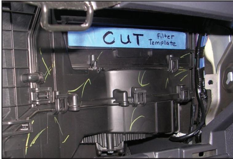
The masking tape template is in place. Time to cut the edges with the "hot butter knife" or Dremel tool.
