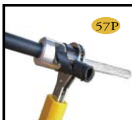
Bugwrench Ratcheting Wire Stripper with Eyeloop Accepts Ripley 4X4 Bushings (Bushing not included) $72.90
